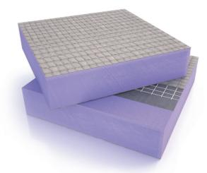
cement coating into which has been bonded a reinforcing fibre glass mesh. This coating provides both excellent point-loading resistance and a superb bond for cement based tile adhesives. Crucially, the whole unit is completely waterproof and dimensionally stable - it is not affected by moisture, humidity or movement in the substrate.
