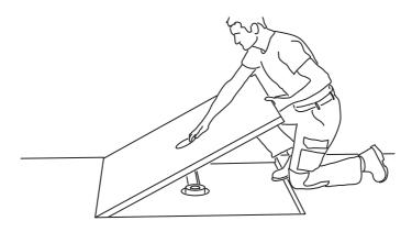
4) The base element is then inserted into the screed recess.
