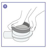
Place the retaining ring with seal ring on the drain unit and push it down firmly until it audibly clicks into place.
