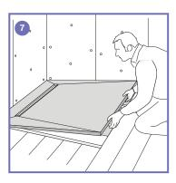
7. Position the shower base over the drain to make sure they are correctly aligned. (But don't remove the protective cover and force the nozzle in to the drain). Ensure any connections created are waterproof at this stage because it will not be possible to return to them once the unit is tiled. (You can do this by pouring water down the drain to check the seals).
