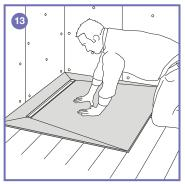
13. Carefully position the Aqua Line Easy shower base over the drain body and push firmly into place, making sure the drain nozzle fits into the seal ring on the drain body. Check that the shower base is level.
