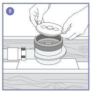
**5.** Cover the floor drain with the protective cover.
